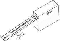
2.3 Pull the tape (printed side up) flat into the trench. ● Place the tape above the buried plastic pipe and keep tape within 4' (1.2m) of final grade.
